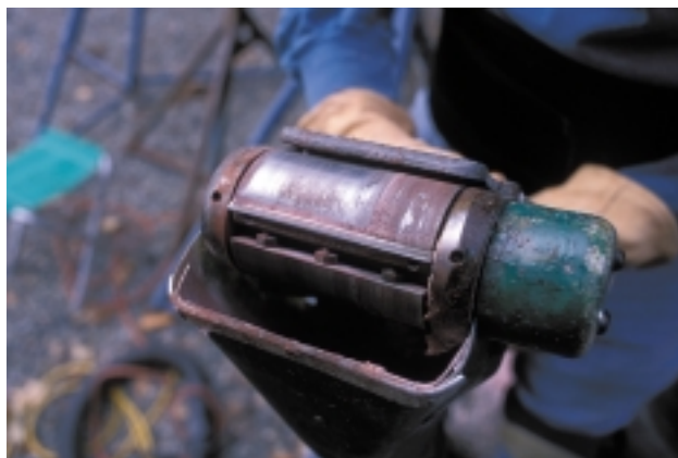
The business end of a fiberglass peeler. The interchangeable blades must be kept sharp for precise cutting.
