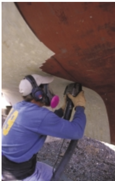
A hull peeler in action. This tool is capable of removing gelcoat and laminate with great precision.
