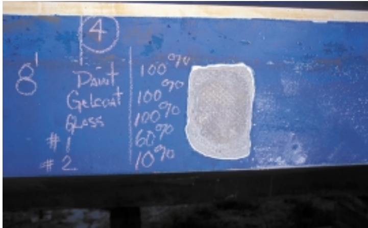
The results of a patch test are written on a hull. The percent symbols seen here are not correct, as all moisture meters read out on a relative scale.
