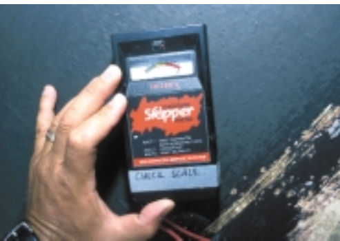
A moisture meter, used by a seasoned professional, is a valuable tool in determining the extent of water saturation in fiberglass. Note, readings taken through antifouling paint are not definitive.
